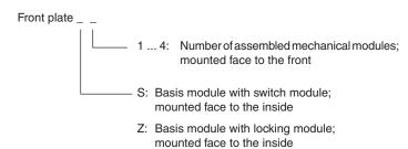
Material: User area: Stainless steel V4A / AISI 316L Mounting plate / front plate to connect and fasten complete functional units of the SAFEMASTER STS modules
